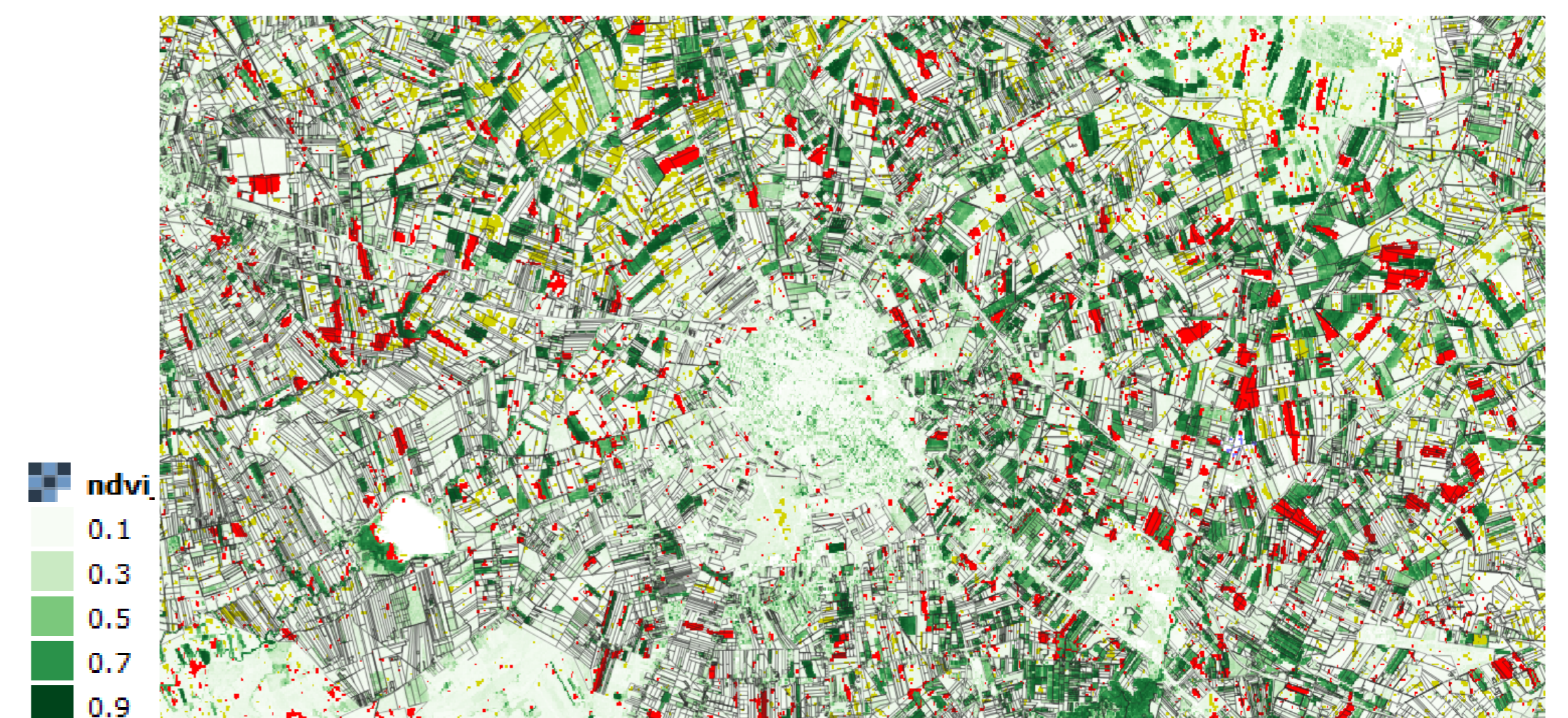
Fig. 1. Map (Apulian Tavoliere, Italy) of temporal changes (between 28 June - 4 July, 2021) of VH polarization S-1 data superimposed on a NDVI S-2 image. Rolled fields are in yellow, plowed fields are in red.
